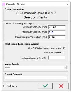
When making water mist calculations and your system meets the criteria which allow Hazen Williams pressure loss formula to be used you can specify a maximum water velocity in the *calculation options* as shown to the left. This dialogue is displayed after you select *calculate*, you can now enter 7.6 m/s as your maximum velocity and if this is exceeded FHC will display a dialogue box at the end of the calculation and will display the pipes exceeding this velocity.
